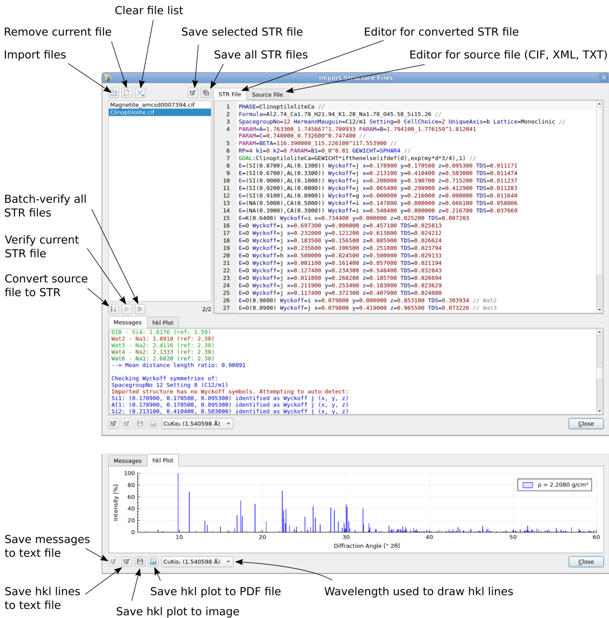
Figure 18: After conversion from CIF to STR format, BGMN will be called in the background to run the STR file. If successful, a hkl stick pattern will be shown, else an error message appears in the „Messages“ page (bottom).
